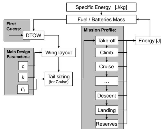
Figure 1 - Scheme featuring the iterative procedure for determining the DTOW, cruise velocity and tail sizing.
