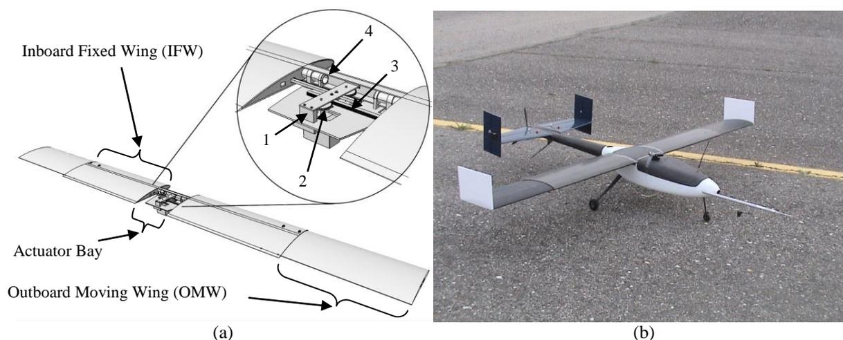
Fig.1 (a) VSW concept: (1) servomotor; (2) transmission pinion; (3) transmission rack; and (4) pultruded carbon spar. (b) UAV fitted with the VSW.
