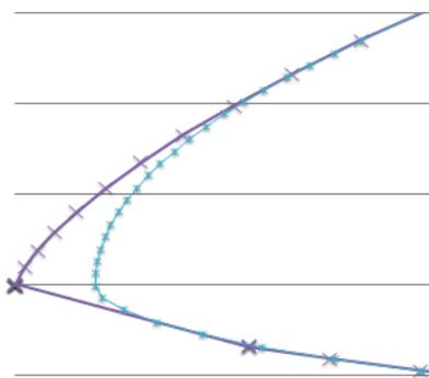
Figure 3 - Double-elliptical function LE curve at the inner offset aerofoil.
