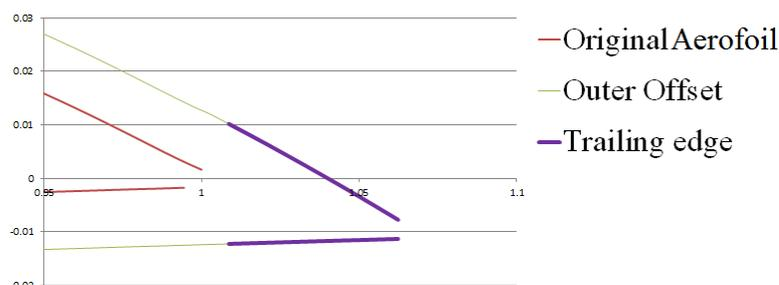
Figure 1 - TE extension at the outer offset aerofoil.
