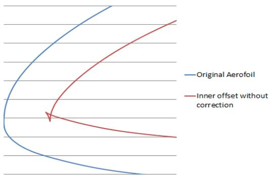
Figure 2 - LE curve at the inner offset aerofoil.
