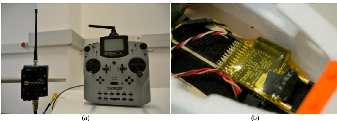
Figure 3- Complete long range radio control system showing: a) the radio controller and the LRS transmitter, and b) the LRS receiver.
