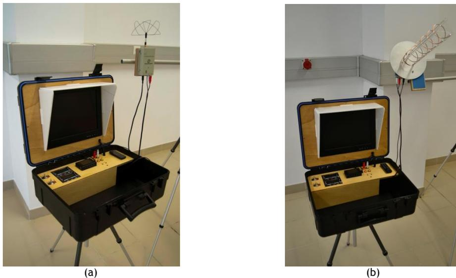
Figure 1- Complete ground control station showing the video receiver connected to: a) skew planar wheel antenna and b) heliaxial high directivity antenna.
