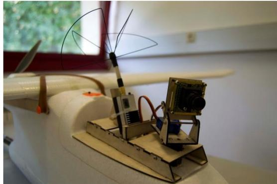
Figure 2-Detachable pod carrying the airborne FPV system components
