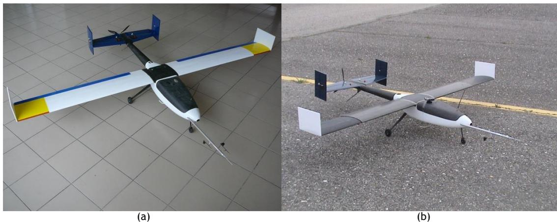
Figure 7-Olharapo UAV fitted with: a) Conventional fixed wing and b) Variable-span wing
